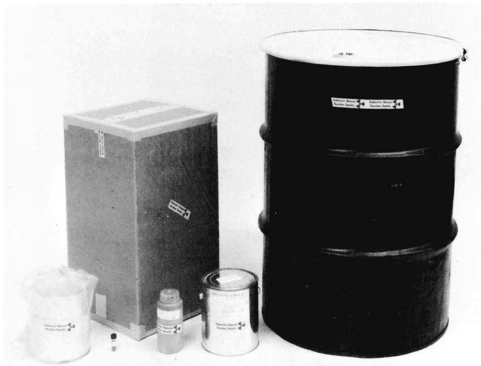
Fig. 1. Examples of containers used for nuclear materials in fuel cycle facilities. The large containers are used for low-concentration scrap and waste, the intermediate-size containers (1- and 4-L) hold high-purity process fuel materials or high-concentration scrap, and the small vial is a typical container for samples withdrawn from process lines for chemical analysis.
