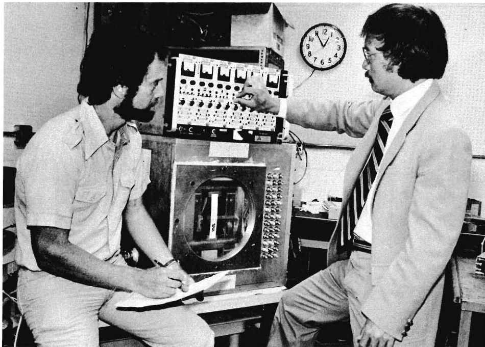
Cy Hoffman (left) and Minh Duong-Van (right) examine a prototype drift chamber, a component of the crystal box detector that will be used to search for rare decays of the muon.
