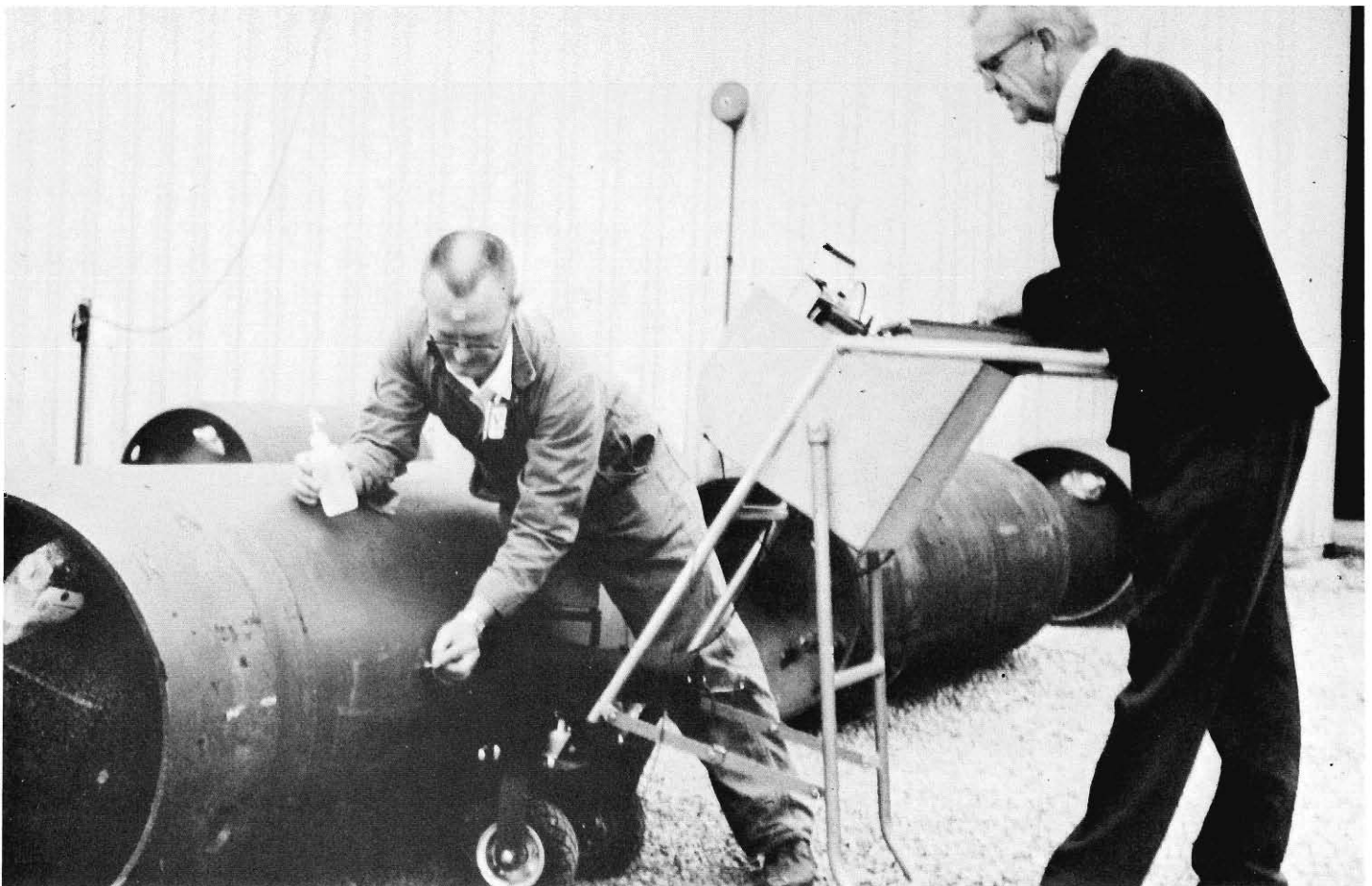
Fig. 10. Field measurement of ^{235}\text{U} enrichment of \text{UF}_6 in a 2-1/2-ton shipping container. A portable NaI detector is used to measure 186-keV ^{235}\text{U} gamma rays. A portable ultrasonic gauge is used to determine the cylinder wall thickness for the attenuation correction.
